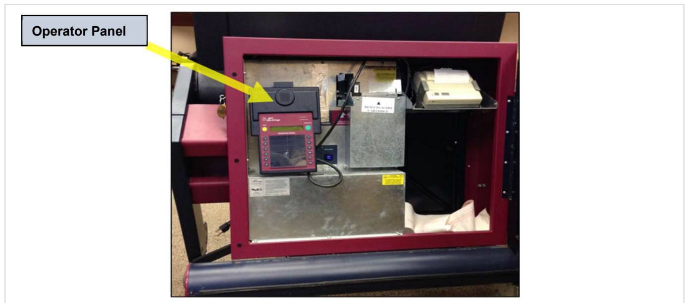
Figure 11: Operator Panel within Back of Unit
