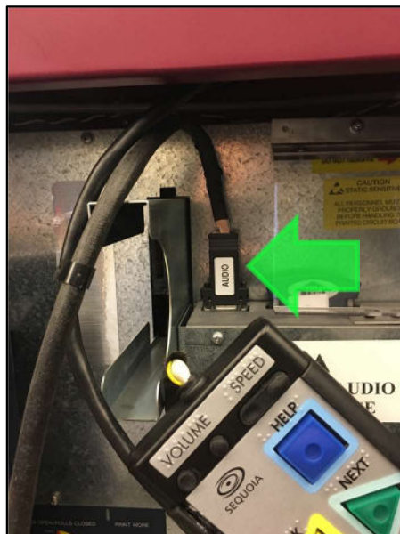
Figure 27: Connect Audio Unit to the Back of the Voting Machine
